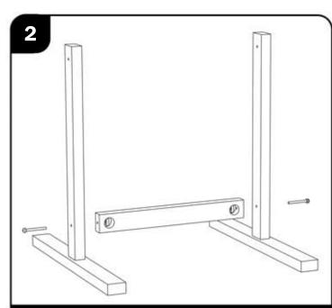
Attach the uprights into the feet using the nuts... Insert the 'V' nuts into the cross member and attach the bolts...
