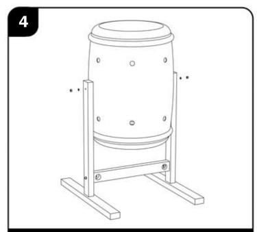
Push the threaded bar through and attach at both ends...
